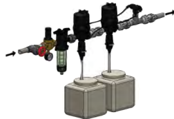
dual remote injection installation
